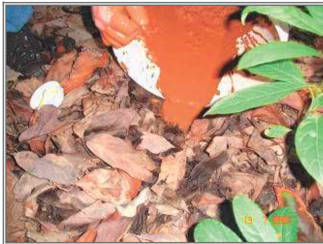
Figure 10: Pouring slurry from the augured hole back into the hole
