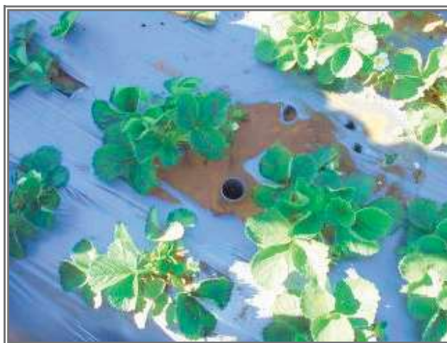
Figure 8: A good fitting access tube
