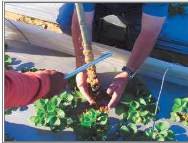
Figure 7: Collecting sand from the augured hole
