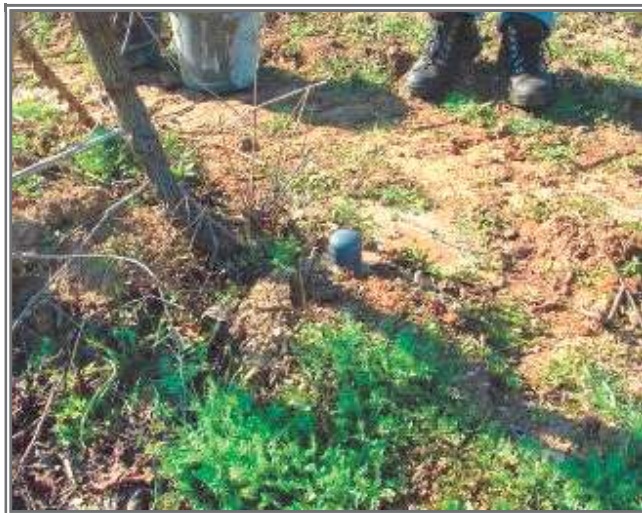
Figure 12: An installed MobiCheck access tube
