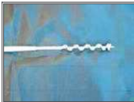
Figure 13: A typical hand-auger bit
