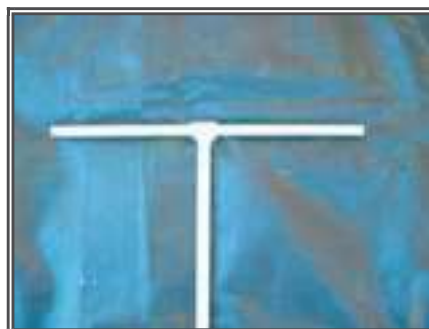
Figure 14: A typical hand-auger T-handle bar
